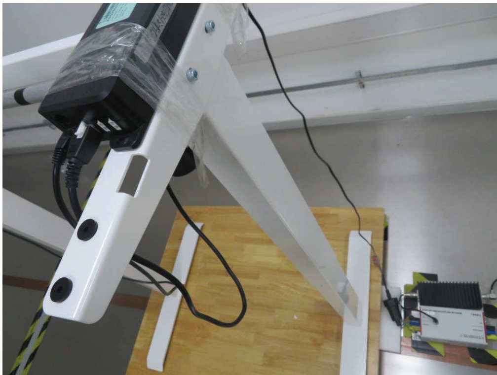
Photograph 6: Setup for Radio-frequency continuous conducted (CS)
